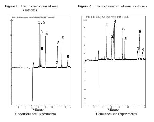
The effects of applied voltage (15 - 30 kV) and temperature (20 - 40°C) on the separation were also studied in the buffer at pH 9.5, which contained 200 mmol/L borate and 10 mmol/L sulfated  $\beta$ -CD. The optimum voltage and temperature were found to be 30 kV and 40°C, respectively, which combined sufficient resolution with a moderate analysis time.
